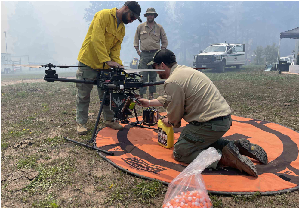
An Unmanned Aerial System (drone) is loaded with plastic spheres that will be dropped into unburned fuels for ignitions at the Spruce Creek fire. (Inciweb photo)
